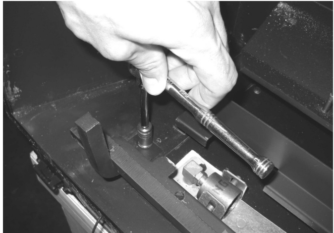
Figure 21. Remove left side Grate assembly M6 nut...
