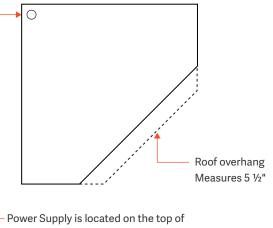
Power Supply is located on the top of the sauna. The cord is approximately 8 feet long.
